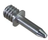
Style "G" guide pin for blind mate applications has #8-32 thread for installation into panel mount HiPer-D connectors with corresponding #8-32 tapped flange. 300 series stainless steel, passivated. One kit consists of (2) guide pins. Install with threadlocking compound. Mates with style "B" guide bushing 289-014-B.
