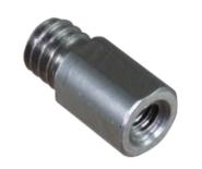
Style "P" jackpost has #8-32 thread for installation into panel mount HiPer-D connectors with corresponding #8-32 tapped flange. 300 series stainless steel, passivated. One kit consists of (2) jackposts. Install with threadlocking compound. Mates with all standard #4-40 male screw locks and jackscrews.
